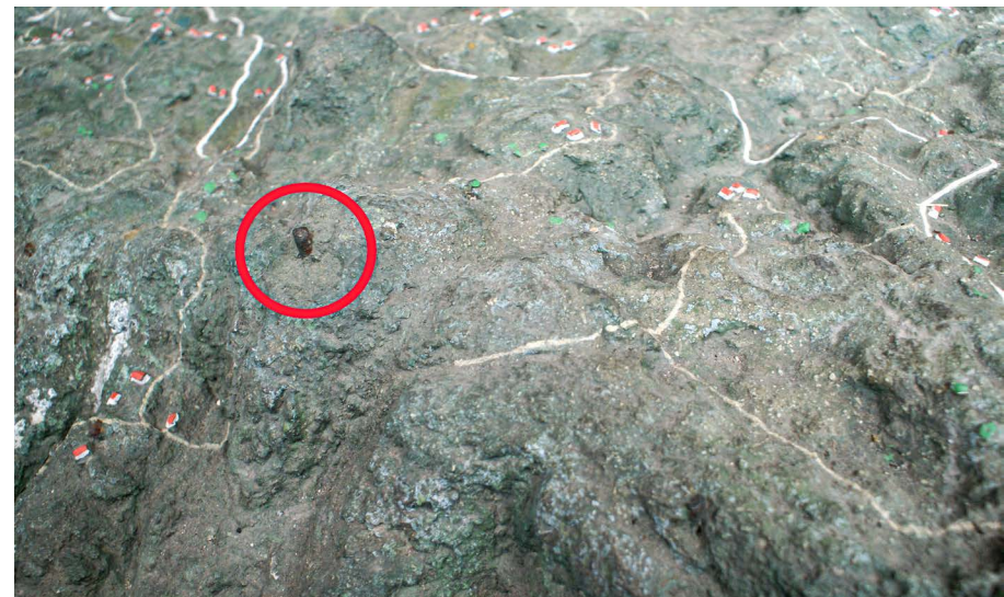
Fig. 10 Example of a Thin Metal Stick for the Determination of Elevation Points, marked with a Red Circle (Mihailo St. Popović, 2020)
